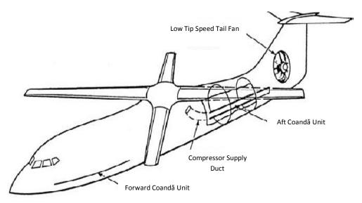
FIGURE 5. X-Wing Configuration and Supply Compressor.
