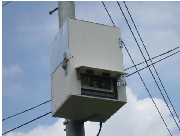
(c) Meteorological data collecting robot (d) Network cameras in the box mounted on the frost damage avoidance pole
